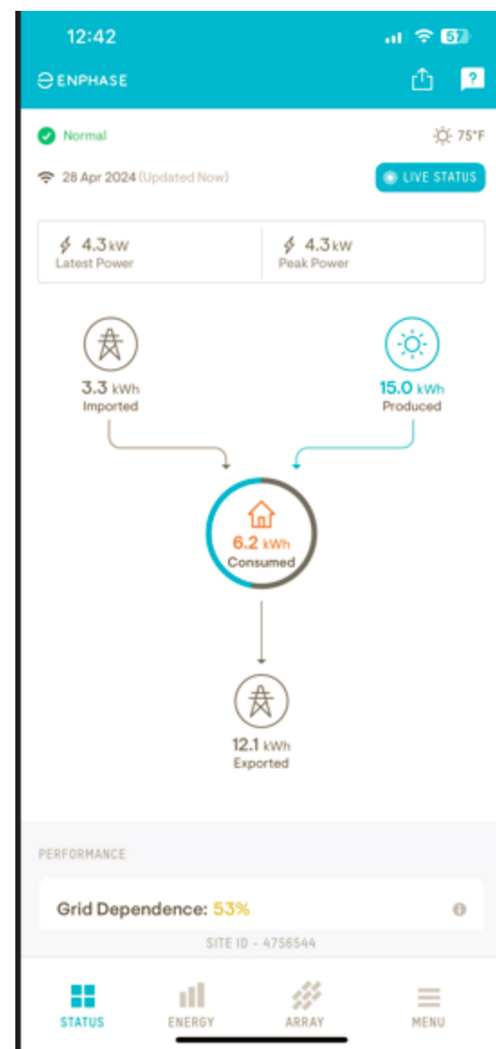
Figure 7. Screenshot from Enlighten app on my iPhone that tracks electricity coming from panels, being used by house, and being put into the grid. It also generates monthly reports and there is a live view option.
